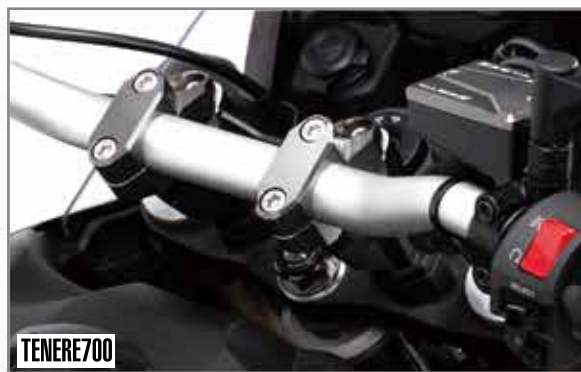
Standard bar 7/8 in ( 22.2 mm )
